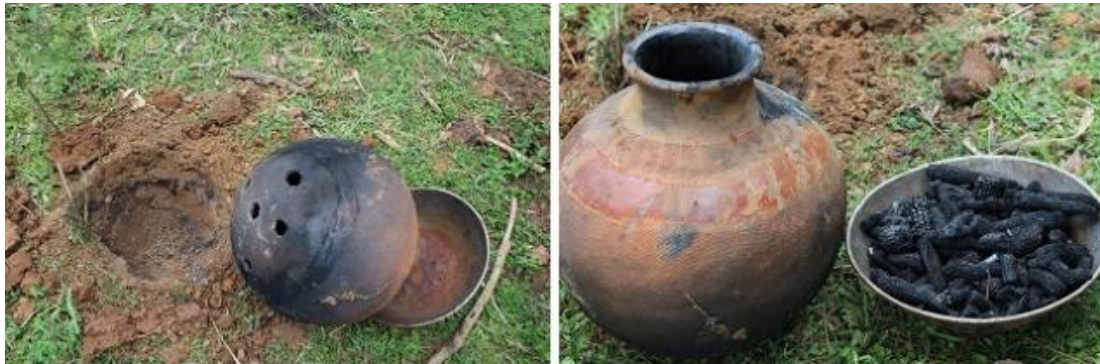
Customized pots for making charcoal out of agricultural waste materials
