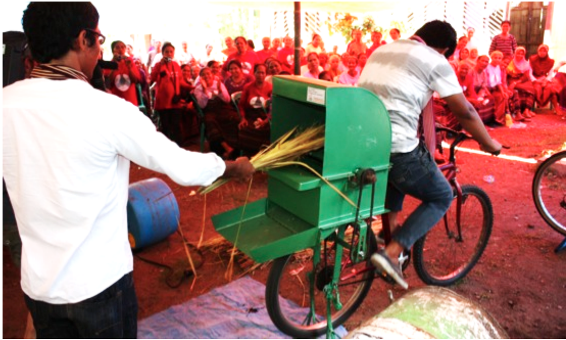
Nengah and Lincoln from Kopernik demonstrating the bicycle-powered paddy thresher in Kelubagolit, East Flores
